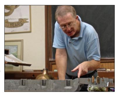
state of the art DRG to spot and drill the holes for the stretchers and horn blocks and then the good old hammer and vice to teach the curvy bits of frame how to behave. Forming a very fine embryo of a five-inch gauge locomotive which will no doubt take two members to lift onto the table at the next WIP.
